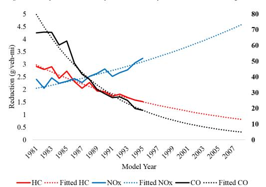
Figure 5: Extrapolated reduction of pollutant for model years 1996-2008. CO is on right axis.
