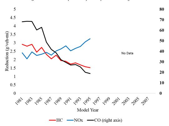
Figure 3: Reduction of pollutant by model year. CO is on right axis.
